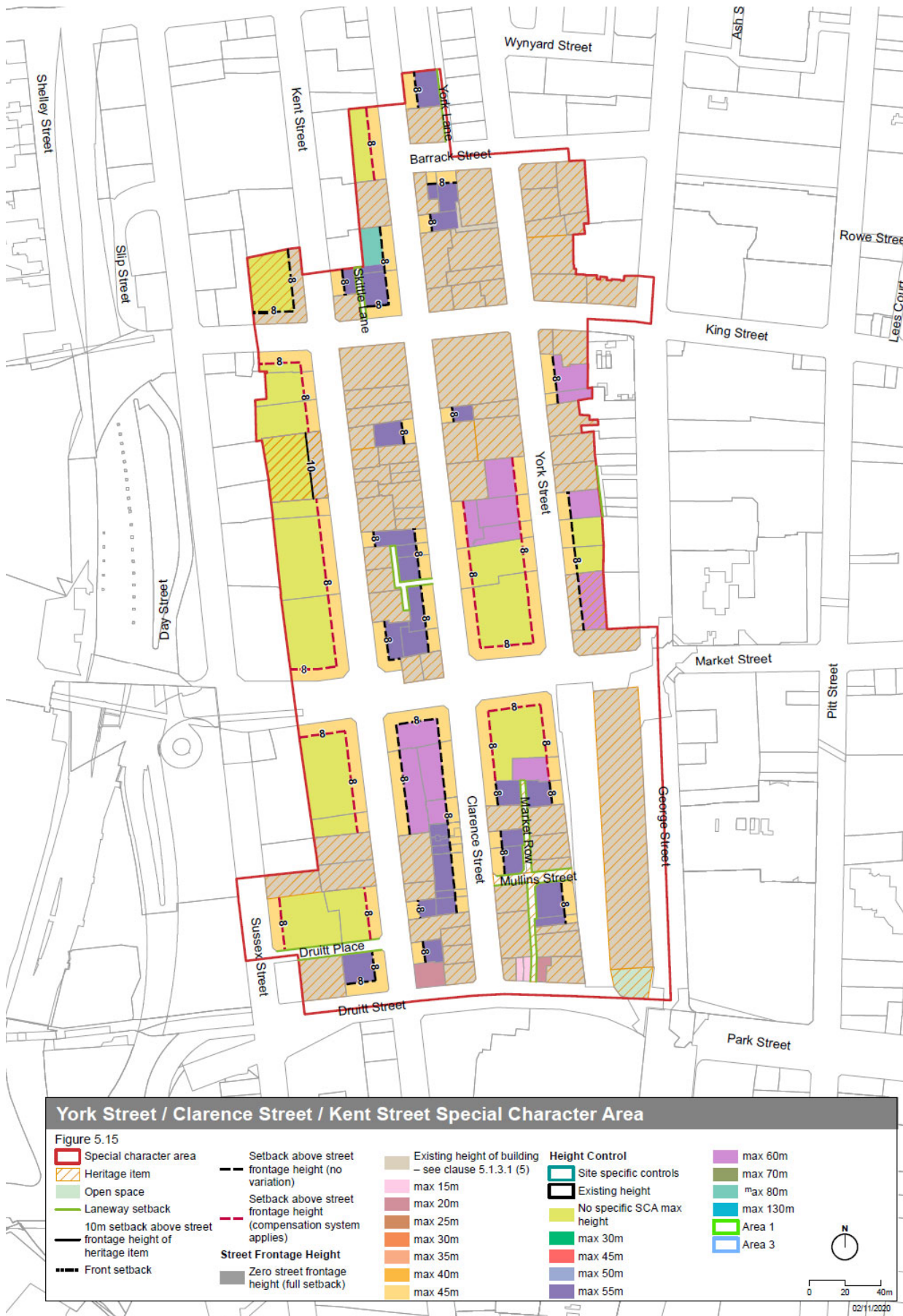
Figure 5.15: York Street/Clarence Street/Kent Street Special Character Area
